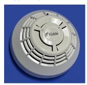
The KC2 Optical Smoke and Heat Combination Detector is a conventional low-profile, self-diagnostic, two-wire photoelectric smoke detector combined with a rate-of-rise and fixed-temperature heat sensor. The advanced photoelectric sensing chamber detects smoke from a fire versus nuisance smoke from non-fire sources. The rate-of-rise heat sensor quickly detects a fast, flaming fire. The fixed-temperature heat
